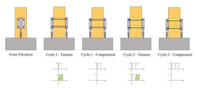
Figure 3. Slack is eliminated on each cycle by the proposed connector, providing a hold-down connection free from pinching.
