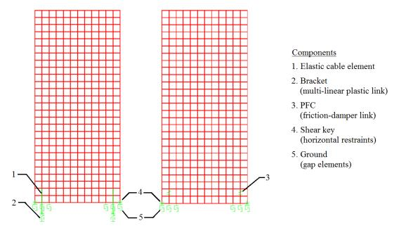
Figure 8. Shear wall models equipped with ordinary bracket connections (left) and pinching-free connections (right).
