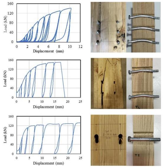
Figure 7. Hysteresis and specimen of the three connections tested. Note that the x-axis scales are adjusted for clarity.
