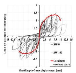
Figure 1. Pinched hysteresis loops observed in typical timber connections [1].
