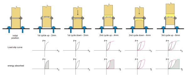
Figure 2. Pinching phenomenon observed in traditional bracket hold-down connectors.
