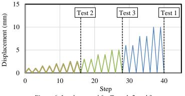
Figure 6. Load protocol for Tests 1, 2 and 3.
