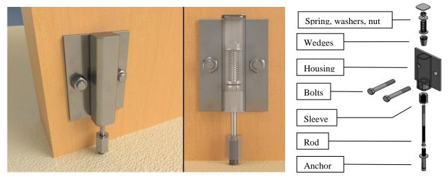
Figure 4. The pinching-free concept applied as a hold-down for rocking shear walls.
